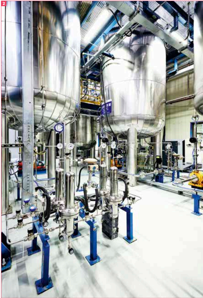
1. The Jiangmen Underground Neutrino Observatory's (JUNO) neutrino detector. Visible on its exterior are the spherical brown Photomultiplier Tubes, 2,400 of which are installed outside the stainless steel structure. Coiled around the sides of the sphere are the Earth Magnetic Field compensation coils. 2. Liquid scintillator mixing vats in the Surface Liquid Scintillator Building. Scintillator is a cocktail of a linear alkylbenzene combined with a solvent.
